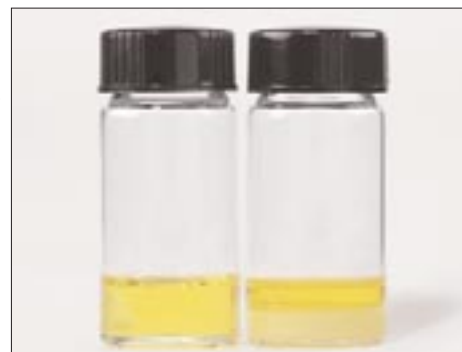
Figure 3. (l) Nanofiller in Adper™ Single Bond 2 Adhesive remains in solution; (r) filler in Optibond Solo Plus™ does not.
