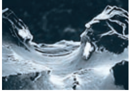
High magnification photo of diamond crystals on a Two Striper® instrument.
