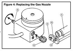
Housing  $\odot$ . Use a 9/16" wrench to unscrew the Gas Nozzle  $\circledcirc$  and replace the old Gas Nozzle with the new Gas Nozzle. Reattach the Burner Assembly to the Valve Housing.
